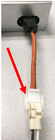
Figure 13: Attach thermostat box to the connector from the switch box.
