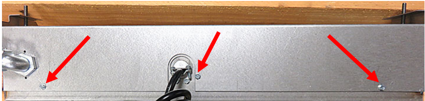
Figure 17: Remove the three sheet metal screws to remove the cover.
