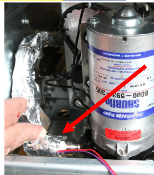
Figure 6: Route the wrapped flex line to the pump inlet side.
