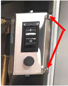
Figure 10: Attach switch box on far right frame next to door.
