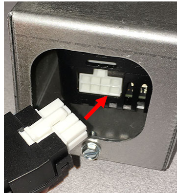
Figure 14: Attach the melter to the thermostat box .
